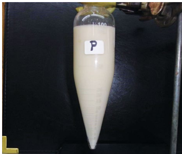
Pan granulated SQUADRON® II formulation in solution one hour after mixing – much better solubility
